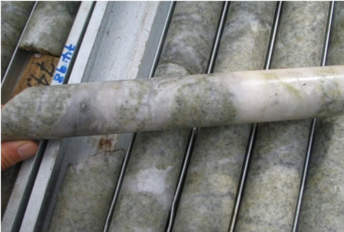
Figure 8-1: Mineralised granite and quartz in diamond core
